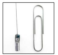
Available as digitally coded tags for the continental MOTUS array and as traditional beeper tags for local movement studies, Lotek produces NanoTags for insects. The latest and lightest NanoTag is the NanoPin, weighing 0.13g. Project managers hope to attach trackers onto any migrating dragonfly species captured, and the smaller NanoPin (image left) will be used on the smaller migrators. This workshop will primarily be for getting a
