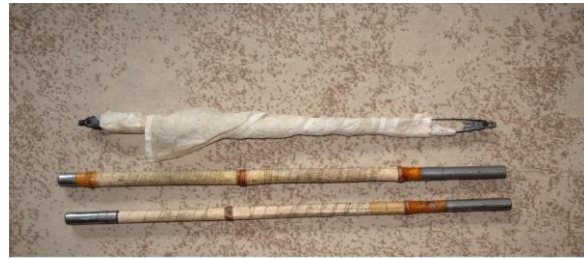
"Harrimac" (? spelling?) folding insect net. Maximum folded lengths = 25 inches Bamboo shaft wound with tape; Aluminum joints; steel net rim. Net when opened = 13 x 15 inches. Assembled net and handle = 64 inches long HarrimacNet2005
